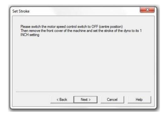
On the control panel on the dyno set the motor speed control switch to the OFF position (centre position). Remove the front cover of the dyno and then change the stroke to 25mm if it is not set already. Replace the front cover and then click 'Next'.
