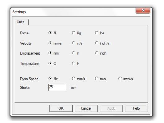
Configure the units when running the dyno calibration. The dyno should be calibrated in its base units i.e. a metric crank dyno should be calibrated in metric. Values can then be converted within the software if required. Leave the dyno speed set in 'Hz' and the stroke value can be left at the stroke value you normally run tests.
