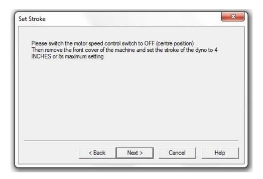
On the control panel on the dyno set the motor speed control switch to the OFF position (centre position). Remove the front cover of the dyno and then change the stroke to 100mm. Replace the front cover and then click 'Next'.
