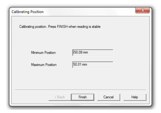
The dyno will now run at 1.0Hz to calibrate the position sensor. Once the maximum and minimum readings stabilise click 'Finish'.
