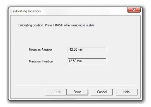
The dyno will now run at 0.5Hz to calibrate the position sensor. Once the maximum and minimum readings stabilise click 'Finish'.
