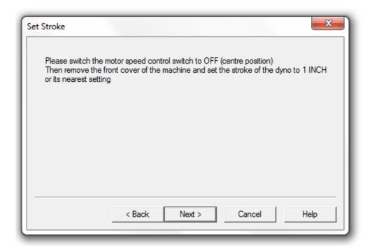
On the control panel on the dyno set the motor speed control switch to the OFF position (centre position). Remove the front cover of the dyno and then change the stroke to 1.0". Replace the front cover and then click 'Next'.
