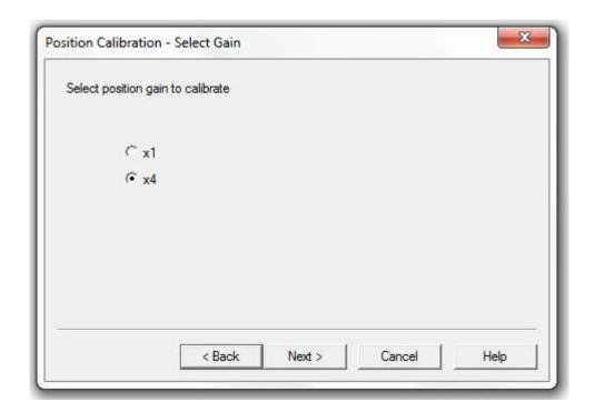
Select x4 position gain to calibrate the position on a 25mm stroke.
