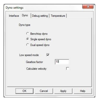
Select 'Single speed Dyno'. Tick 'Low Speed mode' put the gearbox factor as '10.00'. When finished click 'OK'.
