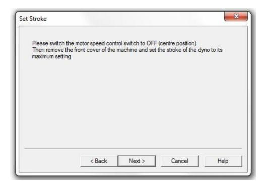
On the control panel on the dyno set the motor speed control switch to the OFF position (centre position). Remove the front cover of the dyno and then change the stroke to 100mm if it is not set already. Replace the front cover and then click 'Next'.
