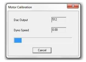
Calibrating the Motor Speed automatically updates the gearbox factor under Configure>System>Dyno.
