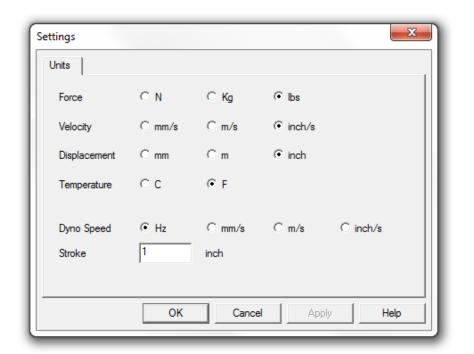
Configure the units when running the dyno calibration. The dyno should be calibrated in its base units i.e. an imperial crank dyno should be calibrated in imperial. Values can then be converted within the software if required. Leave the dyno speed set in 'Hz' and the stroke value can be left at the stroke value you normally run tests.
