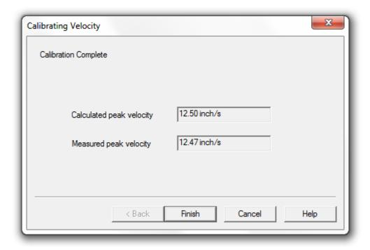
The dyno will now run through the 10 calibration points up to the maximum speed entered. Once this is completed click 'Finish'.
