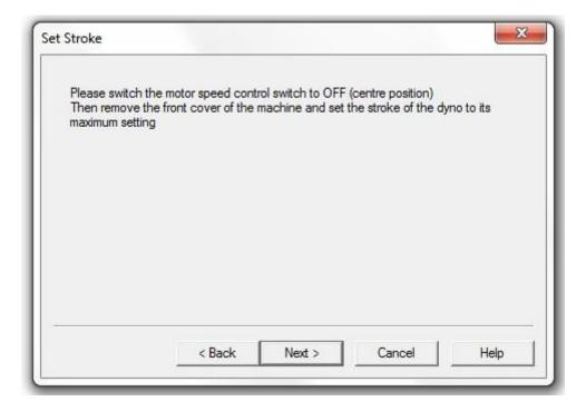
On the control panel on the dyno set the motor speed control switch to the OFF position (centre position). Remove the front cover of the dyno and then change the stroke to 1.0" if it is not set already. Replace the front cover and then click 'Next'.
