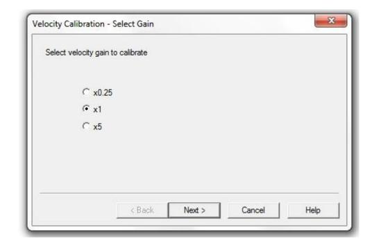
To calibrate the velocity on a 1" stroke select the x1 velocity gain and click 'Next'.
