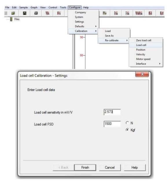
Enter the load cell sensitivity value in mV/V – this value can be found in the folder supplied with the dyno or on a sticker on the load cell. Then enter the load cell FSD – this is the load cell rating which is usually 1500 Kgf for standard load cells. Once the data has been entered click 'Finish'.
