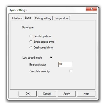
Select 'Benchtop Dyno'. Tick 'Low Speed mode' put the gearbox factor as '10.00'. When finished click 'OK'.
