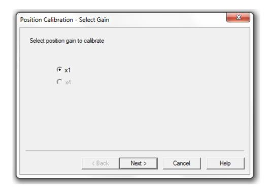
Select x1 position gain to calibrate the position on a 1.0" stroke.
