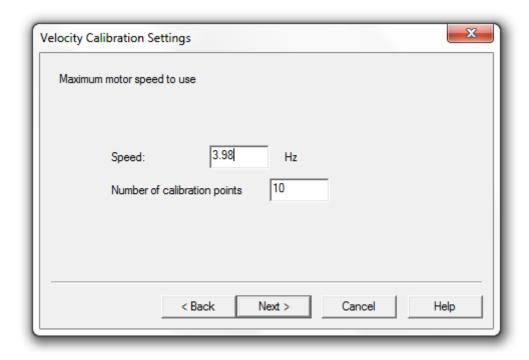
The x1 velocity gain calibrates the sensor in the 0-12.5in/s velocity range. Enter a value of 3.98Hz to give a maximum velocity of 12.5in/s. Enter '10' for the number of calibration points and then click 'Next'.
