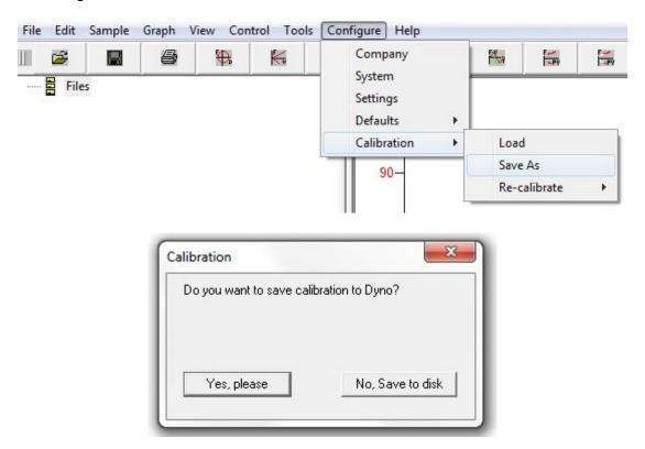
You can save the calibration directly to the dyno interface memory or save it to the PC. We recommend saving it to the dyno and keeping a copy on the PC.
