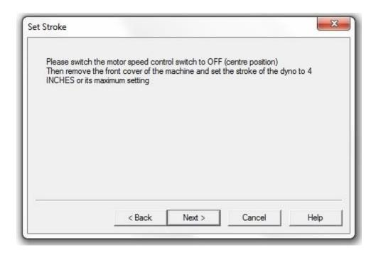
On the control panel on the dyno set the motor speed control switch to the OFF position (centre position). Remove the front cover of the dyno and then change the stroke to 50.0mm. Replace the front cover and then click 'Next'.
