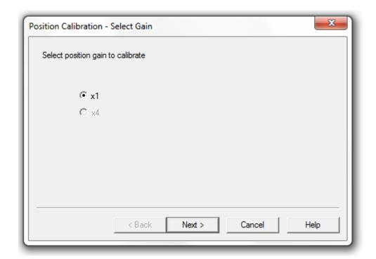
Select x1 position gain to calibrate the position on a 50.0mm stroke.
