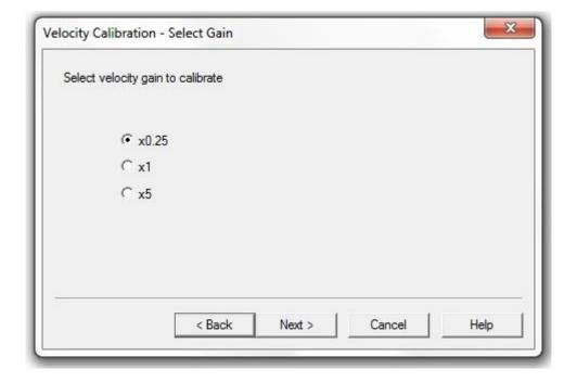
To calibrate the velocity on a 50.0mm stroke select the x0.25 velocity gain and click 'Next'.
