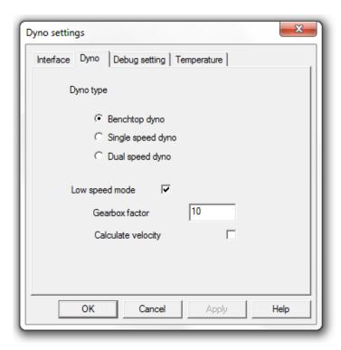
Select 'Benchtop Dyno'. Tick 'Low Speed mode' put the gearbox factor as '10.00'. When finished click 'OK'.
