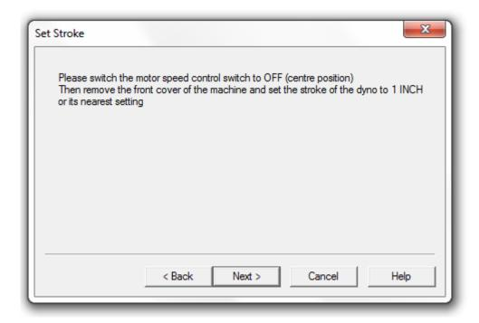
On the control panel on the dyno set the motor speed control switch to the OFF position (centre position). Remove the front cover of the dyno and then change the stroke to 25.0mm. Replace the front cover and then click 'Next'.
