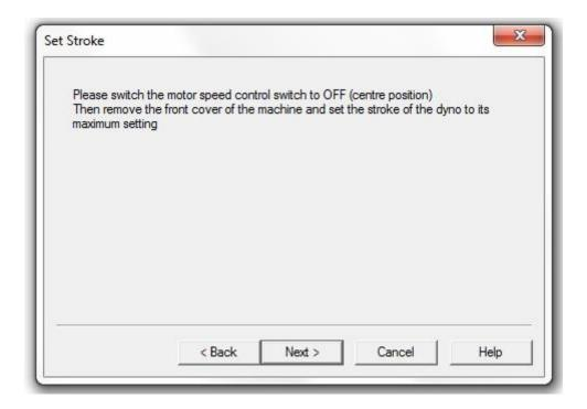
On the control panel on the dyno set the motor speed control switch to the OFF position (centre position). Remove the front cover of the dyno and then change the stroke to 50.0mm if it is not set already. Replace the front cover and then click 'Next'.
