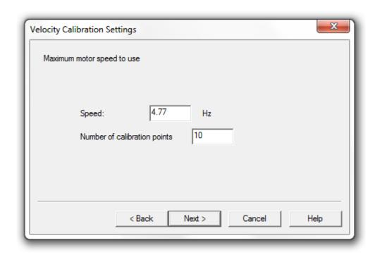
The x0.25 velocity gain calibrates the sensor in the 0-750mm/s velocity range. Enter a value of 4.77Hz to give a maximum velocity of 750mm/s. Enter '10' for the number of calibration points and then click 'Next'.
