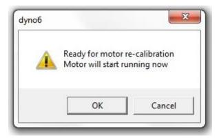
A warning window will open telling you that the motor is going to run. Click 'OK' and the motor speed calibration will start. When the calibration is complete the window will close.
