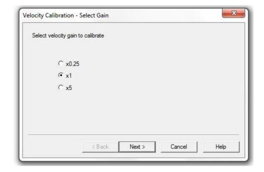
To calibrate the velocity on a 25.0mm stroke select the x1 velocity gain and click 'Next'.
