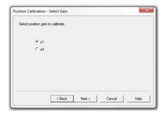
Select x1 position gain to calibrate the position on a 100mm stroke.
