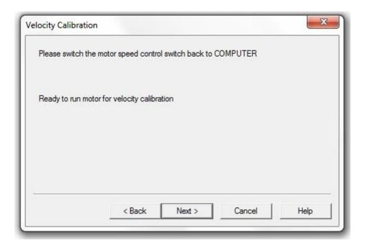
On the dyno control panel switch the motor speed control switch to the COMPUTER position and then click 'Next'.
