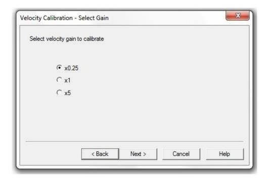
To calibrate the velocity on a 100mm stroke select the x0.25 velocity gain and click 'Next'.
