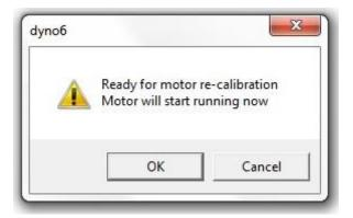
A warning window will open telling you that the motor is going to run. Click 'OK' and the motor speed calibration will start. When the calibration is complete the window will close.
