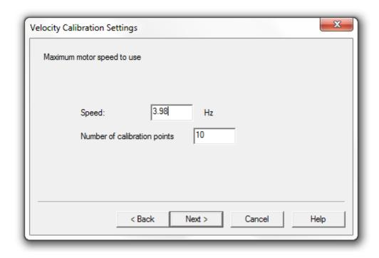
The x1 velocity gain calibrates the sensor in the 0-312.5mm/s velocity range. Enter a value of 3.98Hz to give a maximum velocity of 312.5mm/s. Enter '10' for the number of calibration points and then click 'Next'.
