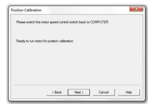
On the dyno control panel switch the motor speed control switch to the COMPUTER position and then click 'Next'.
