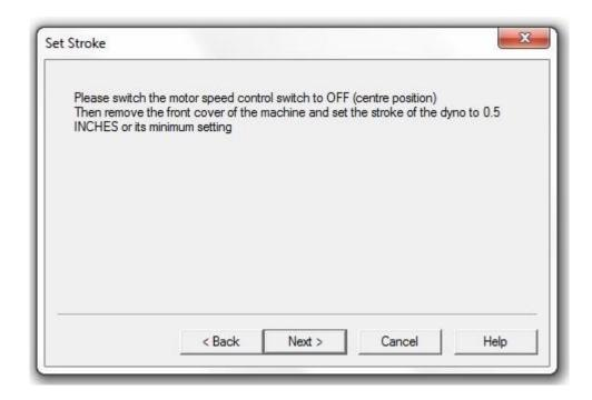
On the control panel on the dyno set the motor speed control switch to the OFF position (centre position). Remove the front cover of the dyno and then change the stroke to 12.5mm. Replace the front cover and then click 'Next'.
