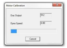
Calibrating the Motor Speed automatically updates the gearbox factor under Configure>System>Dyno.
