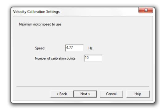
The x0.25 velocity gain calibrates the sensor in the 0-1500mm/s velocity range. Enter a value of 4.77Hz to give a maximum velocity of 1500mm/s. Enter '10' for the number of calibration points and then click 'Next'.
