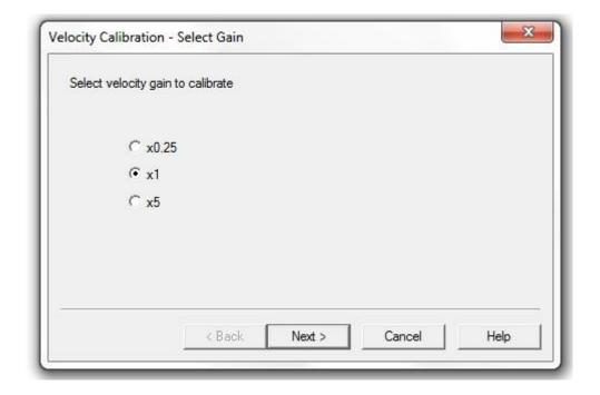
To calibrate the velocity on a 25mm stroke select the x1 velocity gain and click 'Next'.
