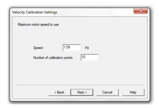
The x5 velocity gain calibrates the sensor in the 0-62.5mm/s velocity range. Enter a value of 1.59Hz to give a maximum velocity of 62.5mm/sin/s. Enter '10' for the number of calibration points and then click 'Next'.
