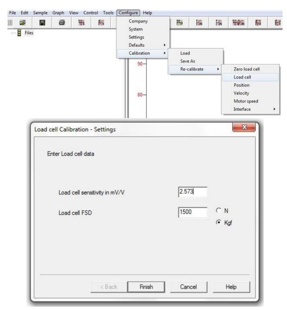
Enter the load cell sensitivity value in mV/V – this value can be found in the folder supplied with the dyno or on a sticker on the load cell. Then enter the load cell FSD – this is the load cell rating which is usually 1500 Kgf for standard load cells. Once the data has been entered click 'Finish'.
