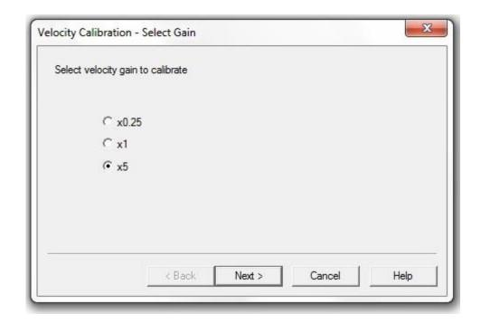
To calibrate the velocity on a 12.5mm stroke select the x5 velocity gain and click 'Next'.
